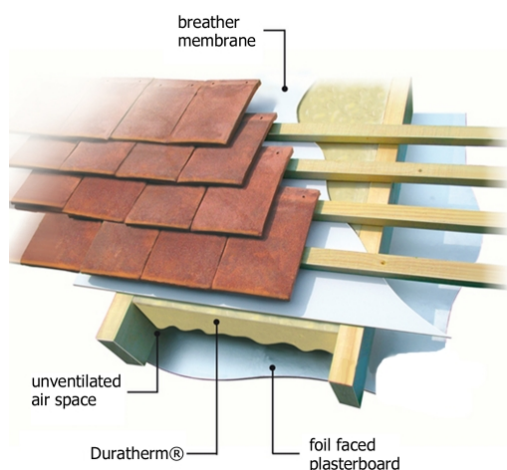
Figure 3 - Warm pitched roof application with insulation covered by plasterboard - habitable roof space
